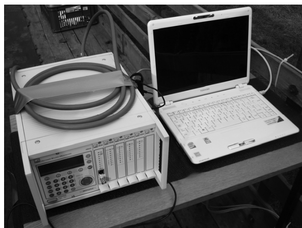
Figure 4. MGC central measurement station connected to a laptop
