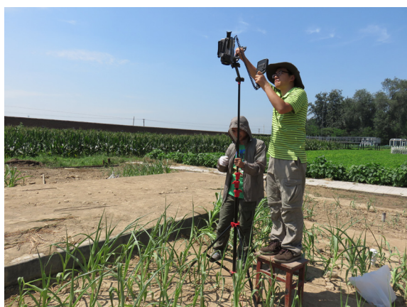
Figure 7. Maize canopy temperature (at 13:30~14:30) measured by the infrared camera (FLIR systems, Therma CAM, P65), revealing higher canopy temperature under drought stress
