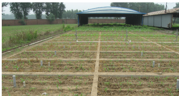
Figure 1. 2 m × 4 m pools cultivating maize, and the electric movable shelter shielding the maize from natural precipitation
